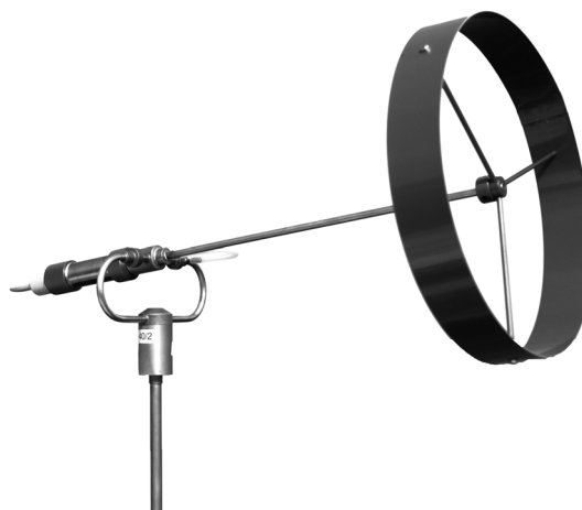
Fig. 3: MINI mounted on a three-dimensional annular-type wind vane for iso-axial sampling
