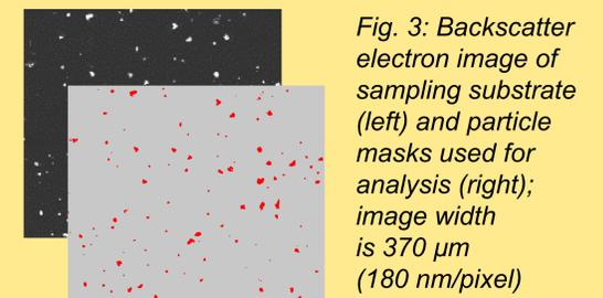
Fig. 3: Backscatter electron image of sampling substrate (left) and particle masks used for analysis (right); image width is 370  $\mu\text{m}$  (180 nm/pixel)
