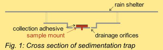
Fig. 1: Cross section of sedimentation trap
